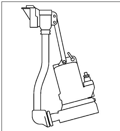
**ATTENTION!** Before fitting the pump, remove any soil, gravel or sand inside the sump.
