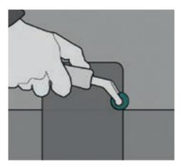
/ Transverse or T-joint connection between two hertalan easy weld roofing sheets can also be realized with a hertalan cover strip.
